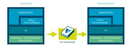
FOX-IT has a number of extra software solutions available that will enhance the value of the Fox DataDiode. These solutions operate at the application level. They include, but are not limited to the Fox DataDiode PI Replicator, the Fox DataDiode Modbus Replicator and the Fox DataDiode OPC Replicator (UA and Classic).
